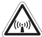
The Above Decks Equipment (ADE) transmits radio frequency (RF) that is potentially harmful. When the system power is ON keep all personnel a minimum of 1.0 m (3.3 ft.) from the antenna (see Radiation Hazard).
